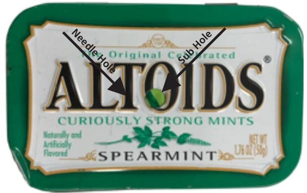
This is what your Pinhole Camera should look like once complete. The larger hole is the sub hole that was drilled. The center is a needle hole punched into a piece of aluminum pop can with a needle hole!
