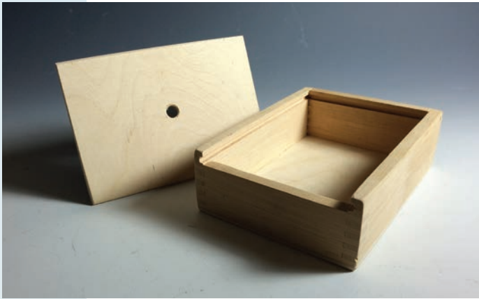
Fig. 1-45. Light-tight box before the interior is painted black.
