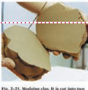
Fig. 2-21. Wedging clay. It is cut into two pieces by use of a tight wire above the wedging table. This is done to examine for air pockets and to better integrate the clay into a homogeneous mass.
